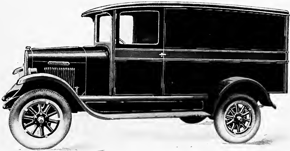
Model 178X De Luxe Bettermetl-Betterwood Panel Body Mounted on International L. D. Chassis
